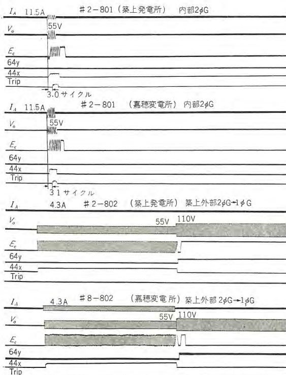
図 2.7 内部 2 \phi G および外部 2 \phi G \rightarrow 1 \phi G オシログラム Fig. 2.7 Oscillograms of test results at two line ground fault for protective zone, and one line ground fault following two line ground fault out of protective zone.
