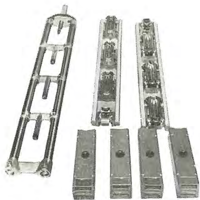
図 4.5 短絡シャ断試験後の接触子 Fig. 4.5 View showing the condition of contacts after the short circuit interrupting test.
