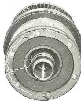
図 3.16 熱電対埋込図 Fig. 3.16 Temperature measurement equipment.
