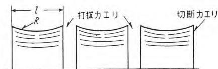
図 3.5 積層鉄心カエリによる変形状態図 Fig. 3.5 Deformed state due to the burr of laminated core.
