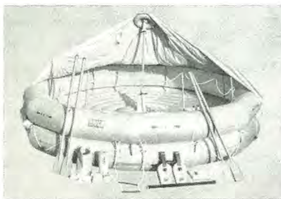
乙形救命イカダの内部構造と付属品 Internal construction of type B life raft and accessories
