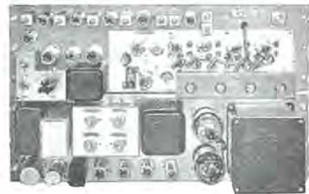
AS-2 形対空無線機受信部, 変調部 Type AS-2 radio equipment (Receiver)
