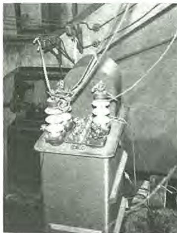
内部温度分布測定中の単器形コンデンサ 417 kVA 3,300 V Tank type capacitor under measurement of internal temperature distribution 417 kVA 3,300 V
