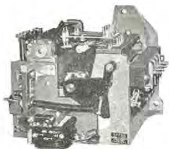
KF-20 形主幹制御器 (ブレーキ制御器) Type KF-20 master controller (for both powering and braking use).
