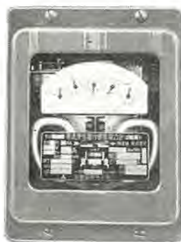
ML-BZ2 形特殊衝流発信装 置付積算電力計 Type ML-BZ2 special bal- anced current watthour meter with transmitter.
