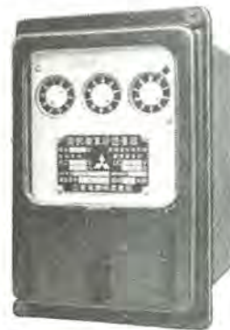
QS-1 形選択積算計送量器 Type QS-1 selective integrated amount transmitter.
