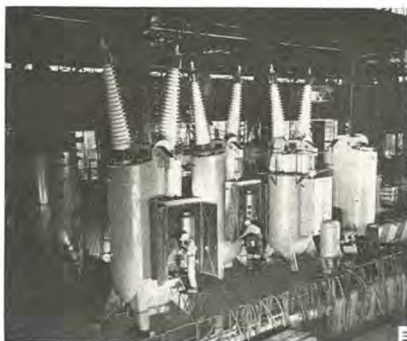
250-GW-1200T 形油シャ断器工場組立中 Type 250-GW-1200T oil circuit breaker.
