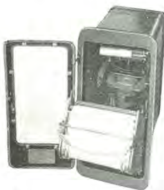
G 形セルシン式記録計内部構造 Interior construction of type G selsyn recorder.
