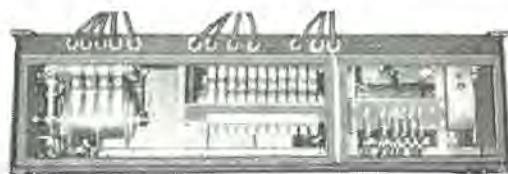
XC-11-112 形カム接触器箱 Type XC-11-112 cam-switch controller box.
