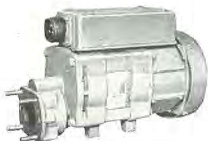
F-86F 用油圧ポンプ用電動機 23 V 0.96 HP 1,800 rpm Alternate hydraulic pump motor for F-86F jet fighter.
