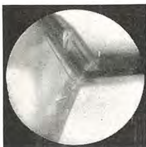
図 4.37 三つ羽根双晶 Fig. 4.37 Twin with three wings.
