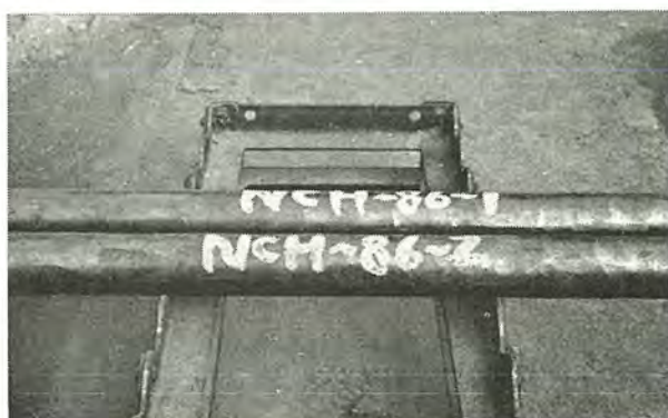
図 4.11 第3回試作再溶解品の鍛造あがりを示す Fig. 4.11 3rd trial remelt after 1st forging.
