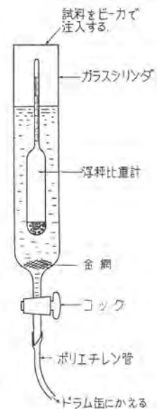
図 4.2 a. 溶剤の比重測定装置 Fig. 4.2 a. Measuring device of specific gravity of solvent.
