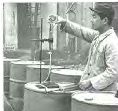
図 4.2 b. 溶剤の比重測定 Fig. 4.2 b. Measuring of specific gravity of solvent.
