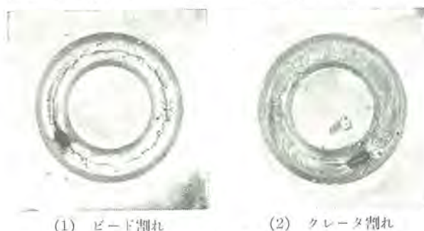
図 3.5 Typical cracks observed in circular-groove tests.
