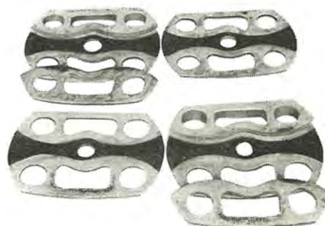
図 4.5 遮断試験後の消弧室ファイバ板 Fig. 4.5 Fiber board of arc extinguishing after interruption test.
