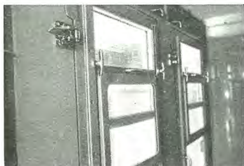
図 4.13 換気調整用窓を閉めた状態 Fig. 4.13 Interior of rectifier car with air tight door shut.
