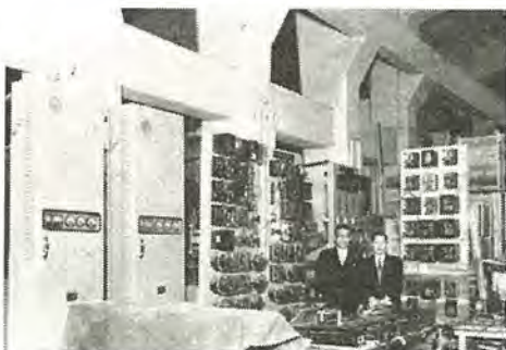
Fig. 3.4 Factory testing device for carrier protective relaying.
