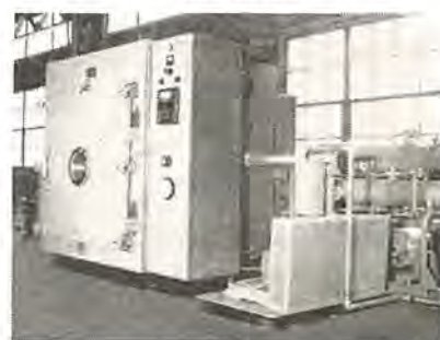
超低温、低圧試験装置 Super low temperature, low pressure testing device.
