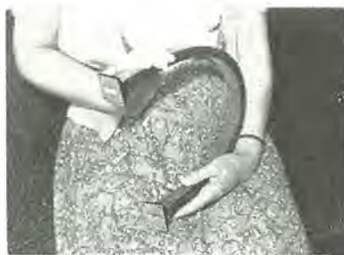
10,000 Mc 帯可撓導波管 Flexible wave guide for 10,000 Mc band.
