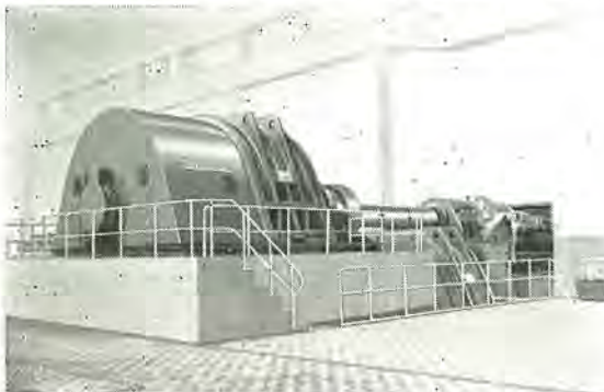
八幡製鉄所厚板ミル用 2×5,000 HP 750 V 40/80 rpm. Twin drive 主電動機 2×5,000 HP Twin drive motor for plate mill.
