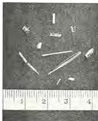
硫化亜鉛単結晶 Zinc sulphide single crystal.
