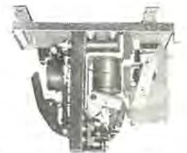
路面電車用高速度断流器中身 High speed line breaker for surface car (content).
