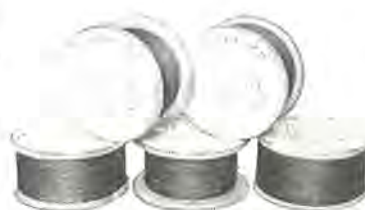
酸化被膜付銅ニッケル抵抗線 Oxide coated copper nickel resistance wire.
