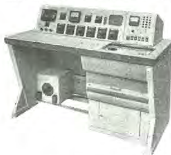
十合百貨店納、拡声 装置調整卓 Mixer console for Sogo department store.
