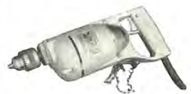
3/8 in 携帯用電気ドリル Portable electric drill.
