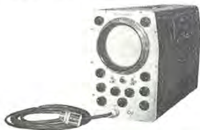
FD 5 型超音波探傷機本体 Type FD 5 supersonic flaw detector.
