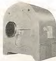
関西電力納誘引通風機用銅冷却管付全閉外扇型屋外型 MKFT 500 kW 3,300 V 60 c/s 10 P Motor for induced draft fan.
