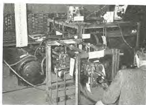
SELD 形ブレーキ装置 10 両編成列車試験台 The train test rack for "SELD" brake equipment (10 car train).
