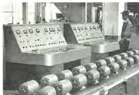
電動機特性試験装置 Motor characteristics testing device.
