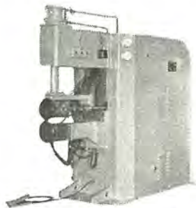
単相シーム溶接機 (30,000 A) Single phase seam welder.
