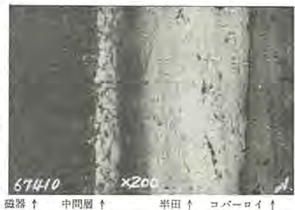
封着部切断面 (200 倍) Cross section of sealed part.
