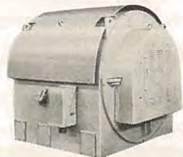
関西電力納誘引通風機用銅冷却管付全閉外扇型屋外型 MKFT 500 kW 3,300 V 60 c/s 10 P Motor for induced draft fan.
