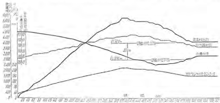
11 図 松神発電所水位調整器試験 Fig. 11. Test record of electric water level regulator for 6,500 kW francis turbine at Matsugami Power Station, Tohoku Denryoku K.K.
