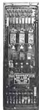
FDS 型継電器 Short cut detection relay.
