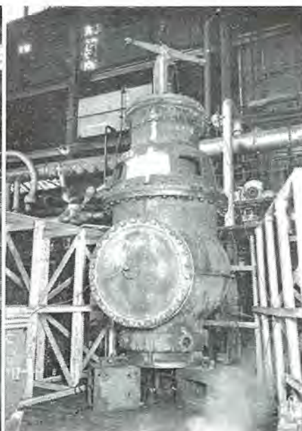
16 図 工場で水圧試験実施中の制圧機 Fig. 16. Pressure regulator on the hydraulic pressure test at factory.
