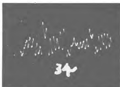
2-5. 短絡環の動作不良を示す. 2-5. Defective short circuitor.
