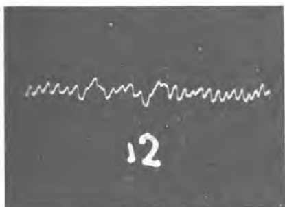
2-2. 写真 2-1 と同一回転子の整流子を短絡環で短絡した場合. 2-2. The same rotor winding with phot. 2-1 when commutator is short circuited by a short circuitor.
