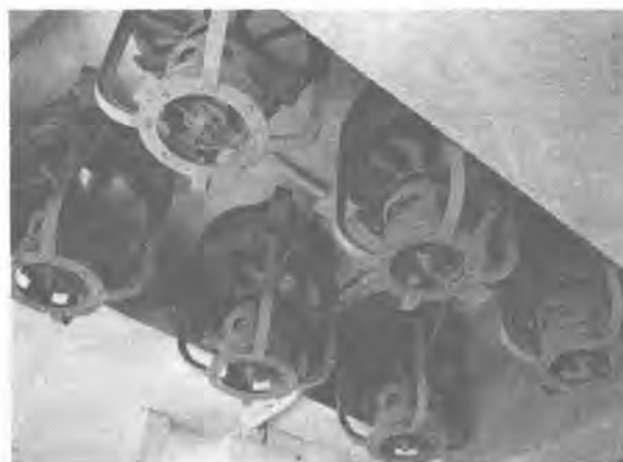
21 図 イグナイトロン冷却扇 Fig. 21. Axial flow type cooling fan mounted on the shaft of a vertical motor.
