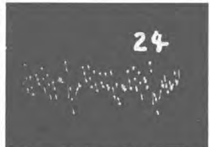
1-10. 同一線輪内短絡2箇所故障。 1-10. Two short circuits between windings in the coil.
