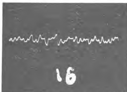
2-3. 整流子を銅線で短絡ライザで数箇所接続不良のもの. 2-3. Rotor with high resistance at several risers when commutator is short circuited by copper wires.
