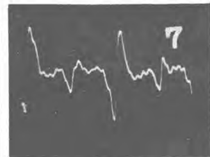
1-11. 線輪端における層間短絡。 1-11. Layer short circuit between coil ends.
