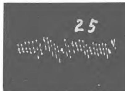
1-8. 同一線輪内1箇所短絡故障。 1-8. A short circuit between winding in the coil.
