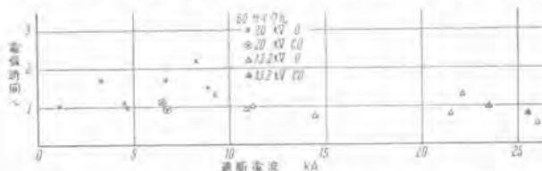
11 図 20-M-100 碍子型遮断器 遮断電流—電弧時間特性 Fig. 11. Type 20-M-100 low-oil-content circuit breaker interrupting current V.S. arcing time characteristic.
