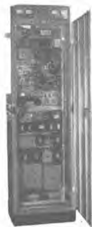
160 Mc 多重無線機 FT-1 Type FT-1 160 Mc multi-channel communication equipment.
