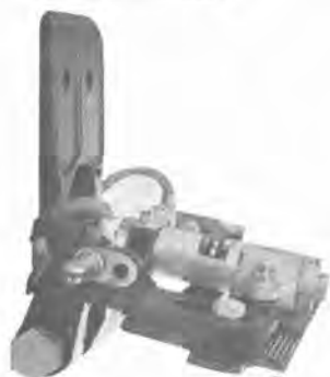
TS-3-A 型集電靴 (側面) "TS-3-A" current collecting shoe. (side view)
