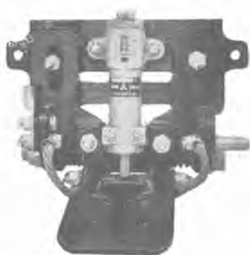
TS-3-A 型集電靴 (正面) "TS-3-A" current collecting shoe. (front view)
