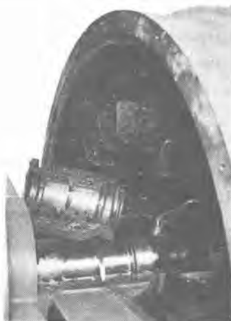
MSF 開放型 1 DM 400 kW 3,000 V 50 c/s 14 P 軸受部 Type "MSF" induction motor 400 kW 3,000 V 50 c/s 14 P 428 rpm cont. rat'g Bearing metal. (Bracket cover removed)
