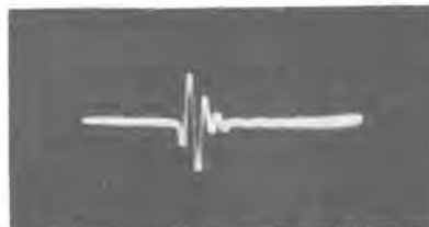
嘉穂の白相着信波形 尖頭値 180 V (線路に接地なき場合 嘉穂 500 Ω 終端) H. F. Pulse received at Kaho white-phase (no grounded point between Takachiho and Kaho, 500 ohm termination at Kaho) received peak value 180 V.
