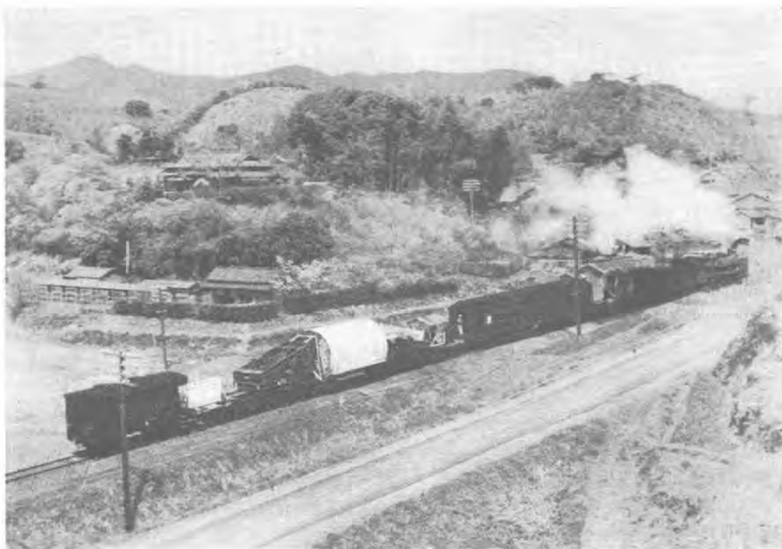
55,000 kW 固定子輸送の実況 55,000 kW rotor in transit.
