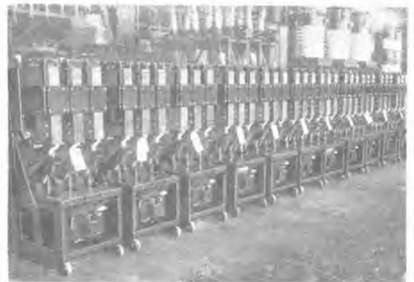
1 図 (b) 量産中の DH 型磁気遮断器 3-DH-15 型磁気遮断器 3,450V 150MVA 1,200A Fig. 1. (b) Type DH magnetic de-ion circuit breakers in mass production (Type 3-DH-15 3,450V 150MVA 1,200A magnetic de-ion circuit breakers).
