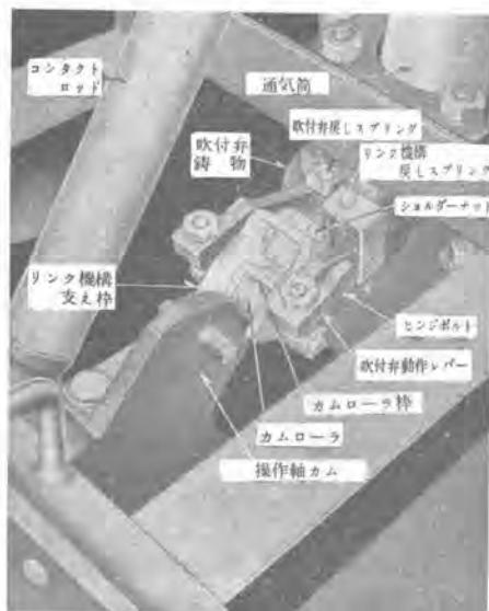
7 図 吹付弁動作機構 Fig. 7. Blowing valve operating mechanism.
