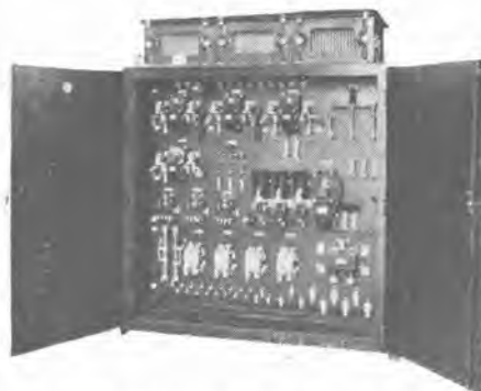
C-12 伸線機 (60 HP) 用制御箱 Control box type C-12 wire drawing machine.
