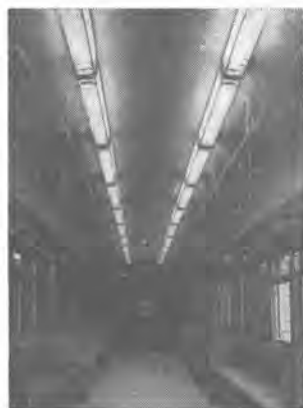
車両用器具 Fluorescent luminaires for car.
