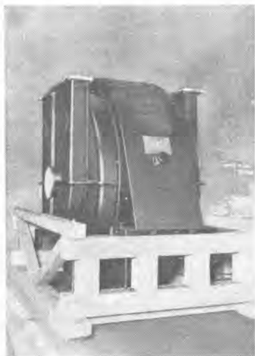
1,500 HP 300 rpm 巻線型閉鎖管通風型誘導電動機 1,500 HP 300 rpm Induction motor for steel mill.
