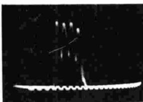
36 図 溶接部探傷波形 (気泡のある箇所) Fig.36. Wave form of the Welded Part. (Where blow holes were found).
